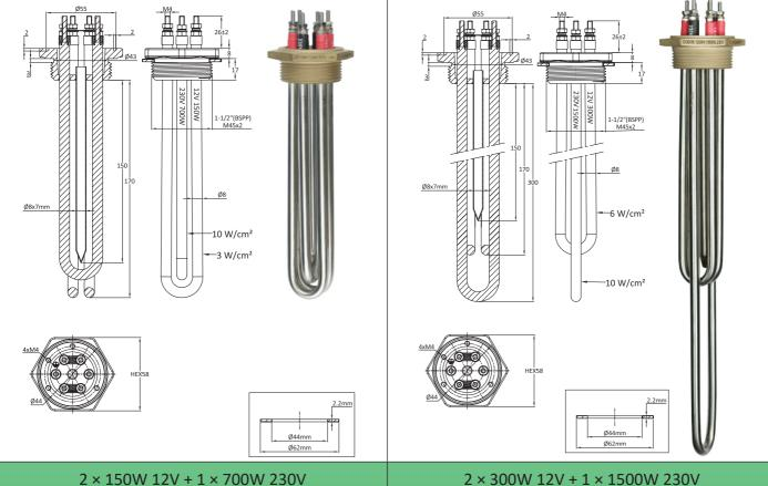
Main application: direct use of low voltage electricity produced by wind turbines or photovoltaic solar panels, for heating liquids, domestic hot water circuits, hot water tanks. These immersion heaters make it possible to use the surplus energy produced, and not used by domestic lighting needs or small electrical appliances. They can also be used in addition to domestic hot water tanks, limiting the need for electricity from the distribution network.
