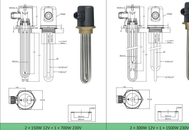
Main application: direct use of low voltage electricity produced by wind turbines or photovoltaic solar panels, for heating liquids, domestic hot water circuits, hot water tanks. These immersion heaters make it possible to use the surplus energy produced, and not used by domestic lighting needs or small electrical appliances. They can also be used in addition to domestic hot water tanks, limiting the need for electricity from the distribution network.
