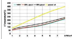
At no flow condition, values of temperature difference 50mm top and 50mm bottom of heating element. It is possible to see huge temperature differences, mainly in oil.
