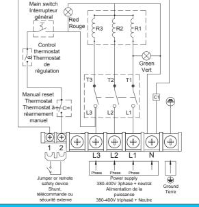
Temperature control thermostat and manual reset thermostat (Types with one heater: phases L1 and L2 are removed, and
