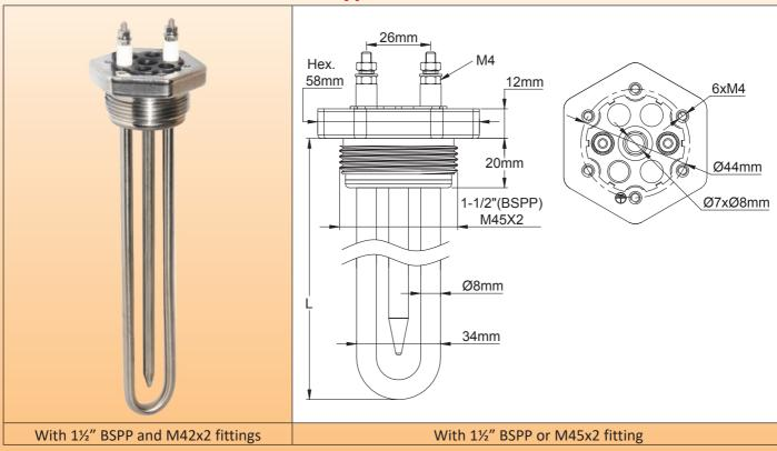
**Main applications:** These immersion heaters with full stainless steel construction are intended for liquid heating applications in scientific, medical, pharmaceutical or food fields, as well as for applications in corrosive environments. All welds are TIG, without any brazing. Liquids are in contact with stainless steel only
