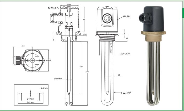
Main application: direct use of low voltage electricity produced by wind turbines or photovoltaic solar panels, for heating liquids, domestic hot water circuits, hot water tanks. These immersion heaters make it possible to use the surplus energy produced, and not used by domestic lighting needs or small electrical appliances. They can also be used in addition to domestic hot water tanks, limiting the need for electricity from the distribution network.
